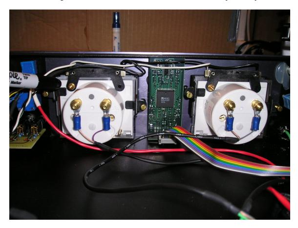
Loosen the nut with a needle nose pliers. Use care as the nut is made of brass and is soft. Remove the lamp holder to expose the bulb. Gently remove the old bulb and replace with a new one.
