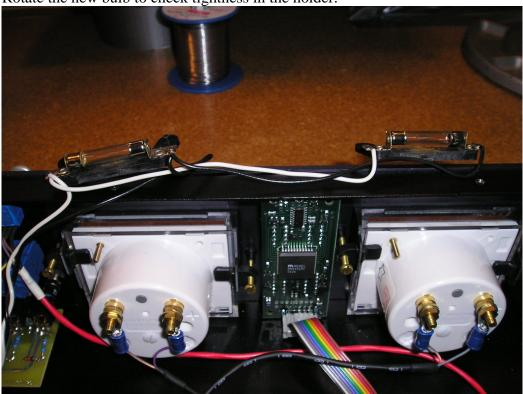
It may be necessary to gently bend the contact springs towards the new bulb to make good contact. To do this, put the new bulb in place and rock the springs towards the center of the holder until the springs grab the bulb tightly.
