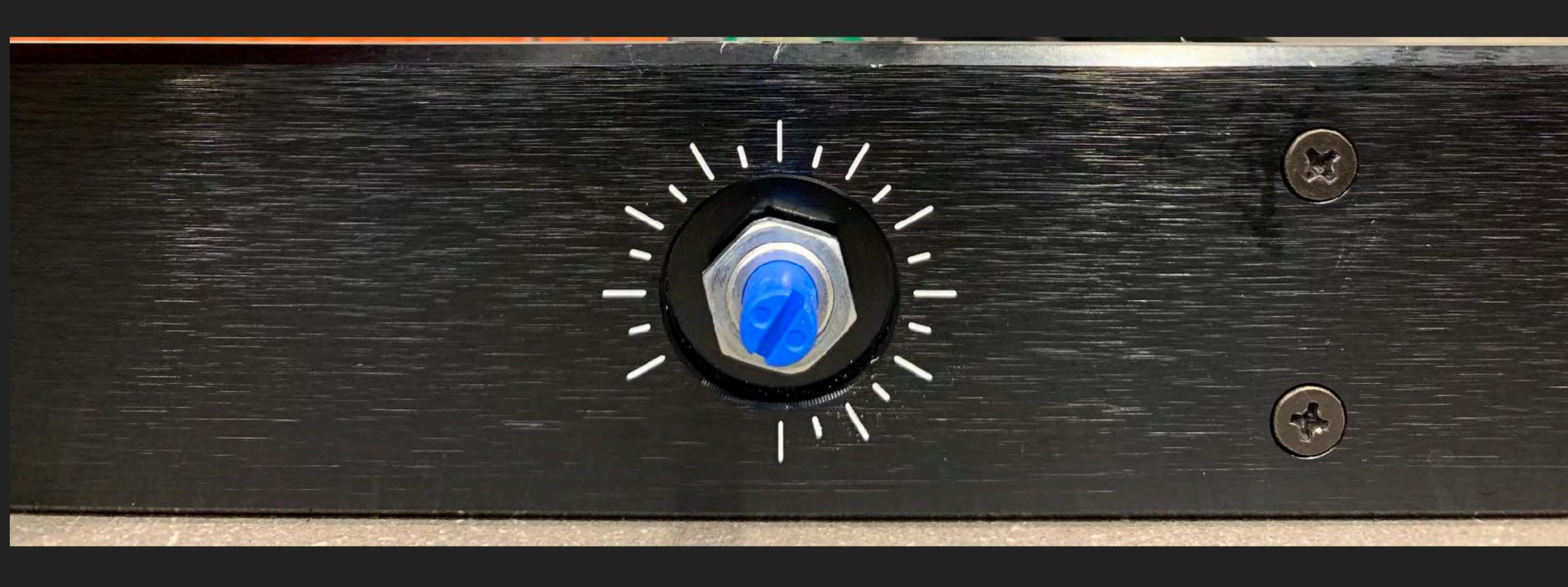
Holding the rear of the pot in place with your fingers, replace the nut
